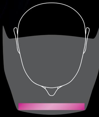
Expanded field of view with a flat filter requires a wider helmet.
